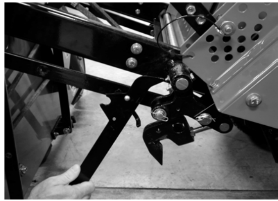
Deck Prop being place against the Deck lift casting
