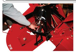
3. Manually push the Safety Catch Channel fully "rearward" until it firmly rests against the cylinder.
