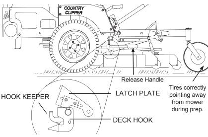
Deck Quick Release System (QRS), right rear deck area
