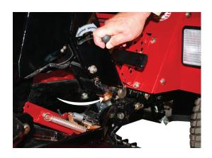
5. Return the Cylinder Locator Arm to the "Mowing" position.
