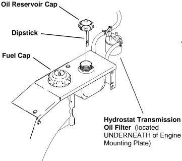
Check the oil level in hydrostatic transmission oil reservoir after every 25 hours of usage. Clean the oil reservoir cap and the area around it prior to removal. Check the oil level on the
