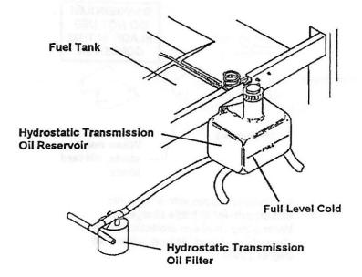
Check the oil level in hydrostatic transmission oil reservoir after every 25 hours of usage. Do not remove the reservoir cap to check the oil level as this allows dirt to enter the transmission. Replenish as needed with 20W-50 Motor Oil.
