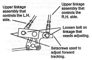
In a large open area, actuate the joystick control lever into the full forward position. If the mower veers to the right, then the right hydrostat needs to be sped up. If it veers to the left, then the left hydrostat needs to be sped up. After determining which hydrostat needs to be sped up, stop the machine, shut off the engine. Slightly loosen the bolt at the lower end of the upper linkage assembly on the side that is slower, and
